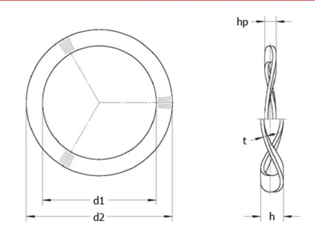
$\begin{array}{ll} d1 &= 39.90 \\ d2 &= 46.00 \\ F(N) \mbox{ at } \mbox{ hp } = 80.0 \\ For \mbox{ bearing } = 6303, \mbox{ } 6005 \\ h &= 3.0 \\ hp &= 1.30 \\ t &= 0.40 \\ Waves &= 4 \end{array}$
